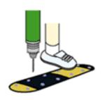
Drill 12MM diameter holes into the surface, through the existing holes of the placed units. The holes should be 120-140MM deep in order to accommodate the plastic shields that are 100MM long.
