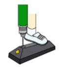
Drill 12MM diameter holes into the surface, through the existing holes of the placed units. The holes should be 120-140MM deep in order to accommodate the plastic shields that are 100MM long.
