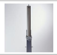
The RetractaPost-GL offers a highly effective and robust way to protect premises and vehicles. The RetractaPost-GL is raised and lowered vertically. When raised the post is 500mm above ground, when lowered the post is fully below ground and covered using the integral lid. The post is lockable in the raised position by rotating the post 45° and then pressing the high-security push button 7-pin security lock. The post is unlocked using the supplied key, rotated and then lowered.
