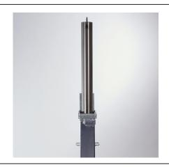
The RetractaPost-GL offers a highly effective and robust way to protect premises and vehicles. The RetractaPost-GL is raised and lowered vertically and is 900mm tall when raised. When lowered the post is fully below ground and covered using the integral lid. The post is lockable in the raised position by rotating the post 45° and then pressing the highsecurity push button 7-pin security lock. The post is unlocked using the supplied key, rotated and then lowered.
