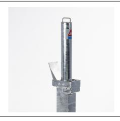
This simple, cost effective, yet highly effective way to prevent unwanted vehicle access. The Post is raised and lowered vertically. When lowered the post is fully below ground and covered using the integral lid. The post is padlockable (padlock not supplied) in the raised position by first rotating the post 45° and then attaching the padlock between the post to the lid. The Post 500 is 500mm above ground in the raised position.
