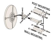
Supplied complete with bolts and brackets kit, adaptable for walls or for posts 60 to 90mm in diameter. Kit is robust, tested to withstand winds of up to 183km/h. Easy to install, allowing precise adjustment of the position of the mirror.
