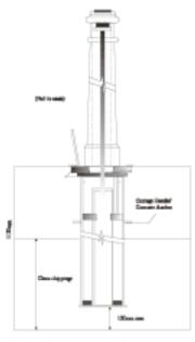
Determine position of installation. Recommended distance between centres: 1250mm, maximum 1400mm.
