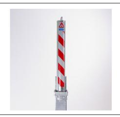
The RetractaPost-GL offers a highly effective and robust way to protect premises and vehicles. The RetractaPost-GL is raised and lowered vertically. When raised the post is 745mm above ground, when lowered the post is fully below ground and covered using the integral lid. The post is lockable in the raised position by rotating the post 45° and then pressing the high-security push button 7-pin security lock. The post is unlocked using the supplied key, rotated and then lowered.
