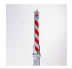
The RetractaPost offers a highly effective and robust way to protect premises and vehicles. The RetractaPost-GL is raised and lowered vertically and is 900mm tall when raised. When lowered the post is fully below ground and covered using the integral lid. The post is lockable in the raised position by rotating the post 45° and then pressing the high-security push button 7-pin security lock. The post is unlocked using the supplied key, rotated and then lowered.
